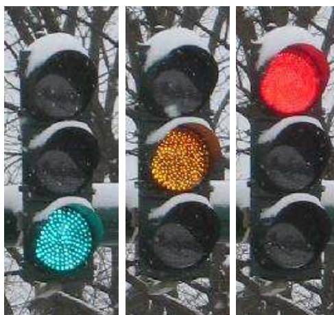
Figure 8.1: Traffic lights in New Haven, CT. The green LED uses InGaN. The red and yellow LED use aluminum gallium arsenide AlGaAs. More recently, aluminum indium gallium phosphide has emerged as a promising material for red, amber, and yellow LEDs.
