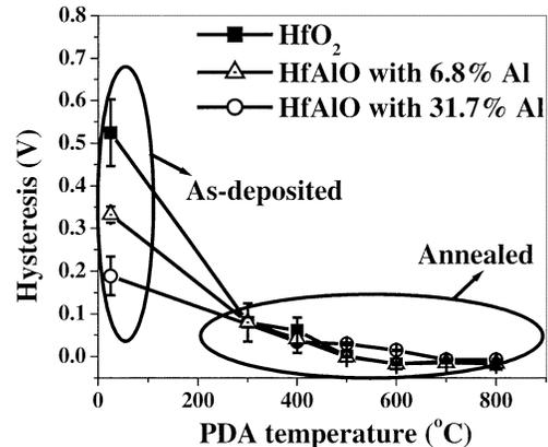
Fig. 5. C-V hysteresis for capacitors made of HfO<sub>2</sub>, HfAlO with 6.8% Al, and HfAlO with 31.7% Al.
