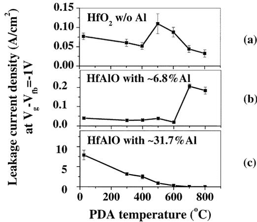
Fig. 2. Gate leakage currents of HfO<sub>2</sub>, HfAlO with ~ 6.8% of Al and HfAlO with ~ 31.7% of Al, as functions of PDA temperature. The EOTs of these films are shown in Fig. 3.
