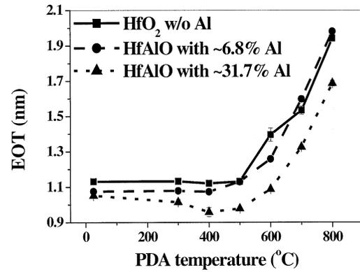
Fig. 3. EOTs of HfO<sub>2</sub>, HfAlO with ~ 6.8% of Al and HfAlO with 31.7% of Al, as functions of PDA temperature.
