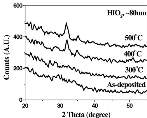
Fig. 1. XRD of HfO<sub>2</sub> after various PDA temperatures.
