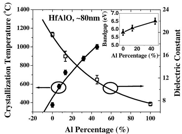
Fig. 4. Crystallization temperature, dielectric constant of HfAlO as functions of Al percentage. The inset shows the band gap of HfAlO as a function of Al percentage.
