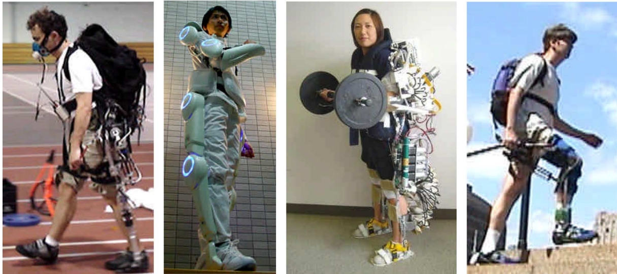
Fig. 5. MIT exoskeleton during metabolic testing [35], HAL-5 exoskeleton [41], nurse-assisting exoskeleton [43], and the RoboKnee [44]. Image credits (from left to right): Prof. Hugh Herr, Biomechanics Laboratory, MIT Media Lab, Cambridge, MA; Prof. Sankai, University of Tsukuba/CYBERDYNE, Inc., Tsukuba, Japan; Prof. Keijiro Yamamoto, Kanagawa Institute of Technology, Atsugi, Japan; Dr. Jerry Pratt, Institute for Human and Machine Cognition, Pensacola, FL.
