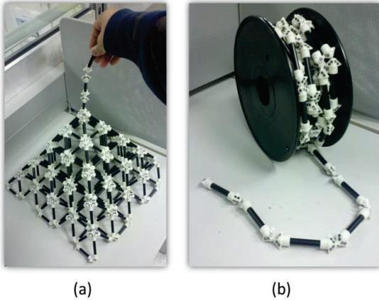
Figure. 1. PICTURES OF OUR PROOF-OF-CONCEPT DESIGN. (a) 293 LINKS ARE USED IN THE FOLDING OF THE PYRAMID SHAPE. (b) A SPOOL OF THE MODULAR CHAIN.
