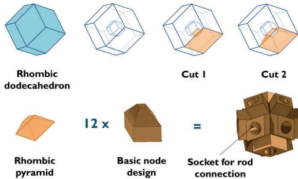
Figure 3. THE FORMATION OF THE BASIC NODE GEOMETRY. *TOP ROW:* A SMALLER RHOMBIC DODECAHEDRON IS FIRST FIT INTO THE CENTER OF THE BUSIEST CONNECTION JOINT. *BOTTOM ROW:* AFTER A SERIES OF CUTTING PROCESS, THE RHOMBIC PYRAMID SHAPE IS SELECTED TO FORM BASIC GEOMETRY OF NODE DESIGN.
