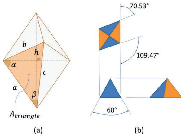
Figure 4. THE IMPORTANT DIMENSIONS OF OUR NODE DESIGN. (a) THE RHOMBIC PYRAMID WITH FOUR SYMMETRICALLY IDENTICAL FACES. (b) SCHEMATIC DRAWING OF THE NODE DESIGN SHOWING THE CRITICAL ASSEMBLY ANGLES.
