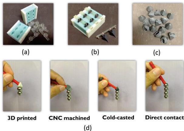
Figure. 9. PROTOTYPING PROCESS OF NODES BY USING COLD-CASTING METHOD. (a) 3D-PRINTED POSITIVES AND THE SILICONE RUBBER MOLD. (b) & (c) COLD-CASTED PARTS MADE FROM THE MIXTURE OF FINE IRON POWDER AND RESINS. (d) COMPARISON OF MAGNETIC FORCES WITH NODES MADE OF DIFFERENT MATERIALS. NOTE: EACH STEEL BALL WEIGHTS 8.4 GRAMS. THE RED ROD IS THE OFF-THE-SHELF GEOMAG PART.
