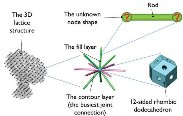
Figure. 2. SCHEMATIC DRAWING SHOWING THE DIFFERENT COMPONENTS AT THE BUSIEST CONNECTION JOINT INSIDE A LARGE THREE-DIMENSIONAL LATTICE STRUCTURE (AN ANTENNA FRAME).
