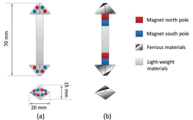
Figure 5. TWO DIFFERENT TYPES OF MAGNETIC COUPLING USED IN OUR PROTOTYPE (a) TYPE-I – EMBEDDING PAIRED MAGNETS DIRECTLY AT THE CONTACTING SITES. (b) TYPE-II – TRANSMITTING MAGNETIC FORCES THROUGH THE NODE MADE OF FERROUS MATERIALS. *NOTE:* THE CENTRAL HOLE IS FOR ANCHORING CONNECTING STRINGS.
