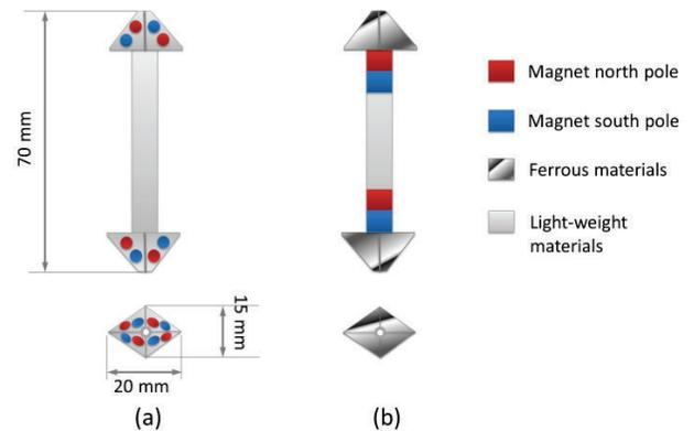
Figure 5. TWO DIFFERENT TYPES OF MAGNETIC COUPLING USED IN OUR PROTOTYPE (a) TYPE-I – EMBEDDING PAIRED MAGNETS DIRECTLY AT THE CONTACTING SITES. (b) TYPE-II – TRANSMITTING MAGNETIC FORCES THROUGH THE NODE MADE OF FERROUS MATERIALS. *NOTE:* THE CENTRAL HOLE IS FOR ANCHORING CONNECTING STRINGS.
