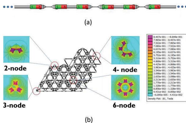
Figure. 7. 2D SIMULATION OF THE MAGNETIC FIELDS BY USING TYPE-II COUPLING METHOD. (a) ALTERNATING THE POLES AT THE TWO ENDS OF EACH ROD. (b) 2D SIMULATION OF THE MAGNETIC FIELDS AT DIFFERENT CONNECTION JOINTS IN A 3D RECONFIGURABLE LATTICE STRUCTURE.
