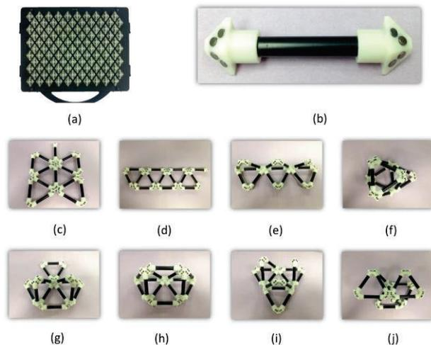
Figure. 8. The PROTOTYPING PROCESS OF NODES VIA 3D PRINTING. (a) A TRAY OF 110 3D-PRINTED NODES. (b) EXAMPLE OF A SEPARATE LINK. (c)-(j) VARIATIONS OF 2D AND 3D STRUCTURES FOLDED BY A 14-LINK CHAIN.
