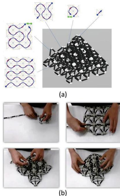
Figure.10. EXAMPLE OF THE FOLDING PROCESS. (a) THE SEPARATE FOLDING PATHS FOR CONSTRUCTING DIFFERENT LAYERS OF A PYRAMID. (b) SNAPSHOTS SHOWING THE DEMONSTRATION OF PLANNED FOLDING PROCESS.
