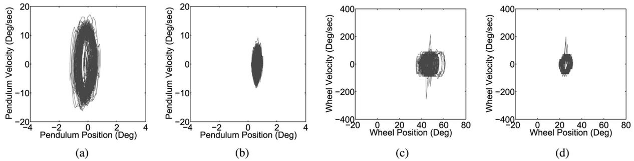
**Fig. 6 Phase plots showing relative stability—(a) pendulum pitch versus pitch rate with hard tires, (b) pendulum pitch versus pitch rate with soft tires, (c) wheel position versus velocity with hard tires, and (d) wheel position versus velocity with soft tires**
