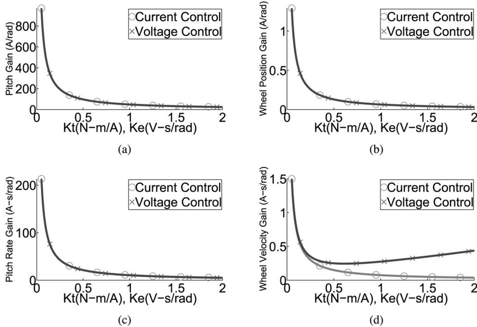
**Fig. 13** (a) Variation of pitch gain with motor constants, (b) variation of wheel position gain with motor constants, (c) variation of pitch rate gain with motor constants, and (d) variation of wheel velocity gain with motor constants. Note: the wheel velocity gain is the only gain that reduces the stability margin of the voltage controlled WIP.
