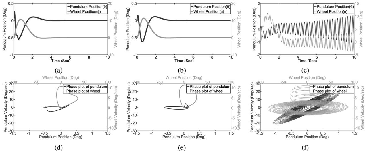
**Fig. 8 Simulated output of WIP response to disturbance of 0.0873 rad/s in pitch rate under the following filter configurations. (a) and (d) Wheel velocity filter  $f_c = 5.0$  Hz and pitch rate filter  $f_c = 5.0$  Hz; (b) and (e) wheel velocity filter  $f_c = 5.0$  Hz and pitch rate filter  $f_c = 50.0$  Hz; (c) and (f) wheel velocity filter  $f_c = 50.0$  Hz and pitch rate filter  $f_c = 5.0$  Hz. Note the instability of the response in plots (c) and (f).**
