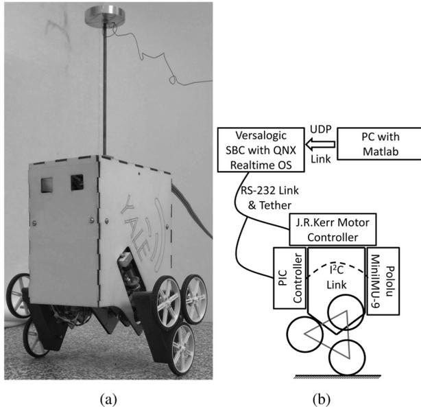
Fig. 2 (a) Charlie—balancing and (b) system architecture
