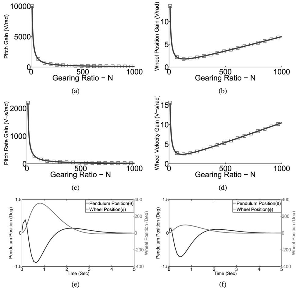
**Fig. 14** (a) Pitch gain variation with gearing ratio, (b) wheel position gain with gearing ratio, (c) pitch rate gain with gearing ratio, (d) wheel velocity gain with gearing ratio, and (e) and (f) simulation of WIP response to a disturbance of 0.1745 rad/s in pitch rate with gearing ratios  $N=50$  and  $N=200$
