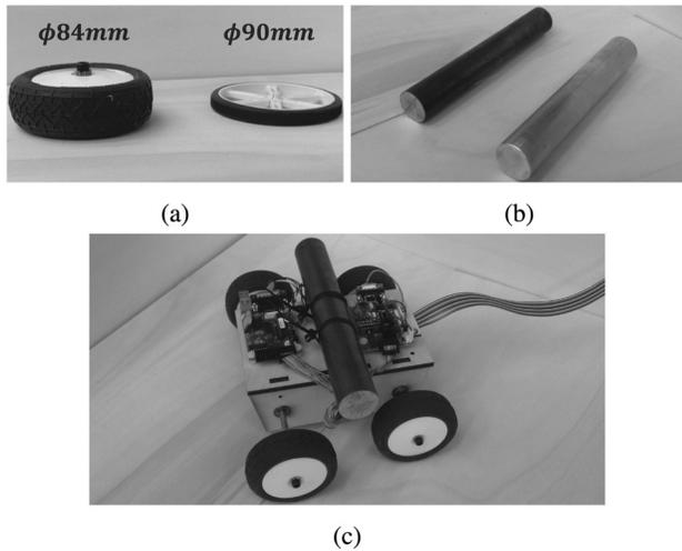
**Fig. 4** Tire testing setup: (a) two tires were tested, 84 mm diameter on left and 90 mm diameter on right; (b) steel and aluminum rods of equal dimensions weighing 0.912 kg and 2.220 kg were loaded on the cart; and (c) cart instrumented with optical encoder to measure position and velocity
