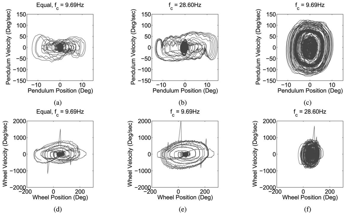
Fig. 9 (a)–(f) Phase plots with various filter configurations, filter cutoffs are indicated: (a) and (d) phase plots with equal cut off frequencies. (b), (e) and (c), (f) Phase plots with different cutoff frequencies.
