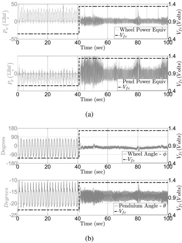
**Fig. 11** Two types of limit cycle behavior depending on the magnitude of the compensation term,  $V_{fc}$ . From 0 to 40 s, the plots display limit cycles generated due to an underestimation of  $V_{fc}$  while from 40 to 100 s limit cycles due to an overestimation of  $V_{fc}$  are displayed. (a) Wheel and pendulum power products. The negative spikes in  $P_w$  and positive spikes of  $P_p$  between 0 and 40 s indicate deviation quadrants IV and III, and (b) pitch and wheel positions.
