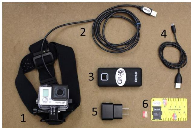
Figure 2: The contents of the equipment ‘kit’ sent to remote participants via postal courier. The contents are as follows: 1. Head strap and GoPro camera with modified case to allow USB connection 2. Long mini-USB cable for connecting GoPro to Power Bank 3. Power Bank 4. Short micro-USB Cable for re-charging Power Bank 5. USB charger 6. Micro SD cards and organizer / holder (the bottom row is for empty cards which are moved to the top row when they contain data).
