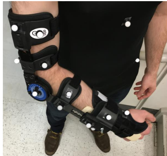
Figure 4. A custom bracing system was created for this study by combining an commercial elbow brace with a wrist orthosis, modified with an additional wooden insert to limit wrist flexion/extension. This arrangement limits motion of all 3DOF of the wrist.
