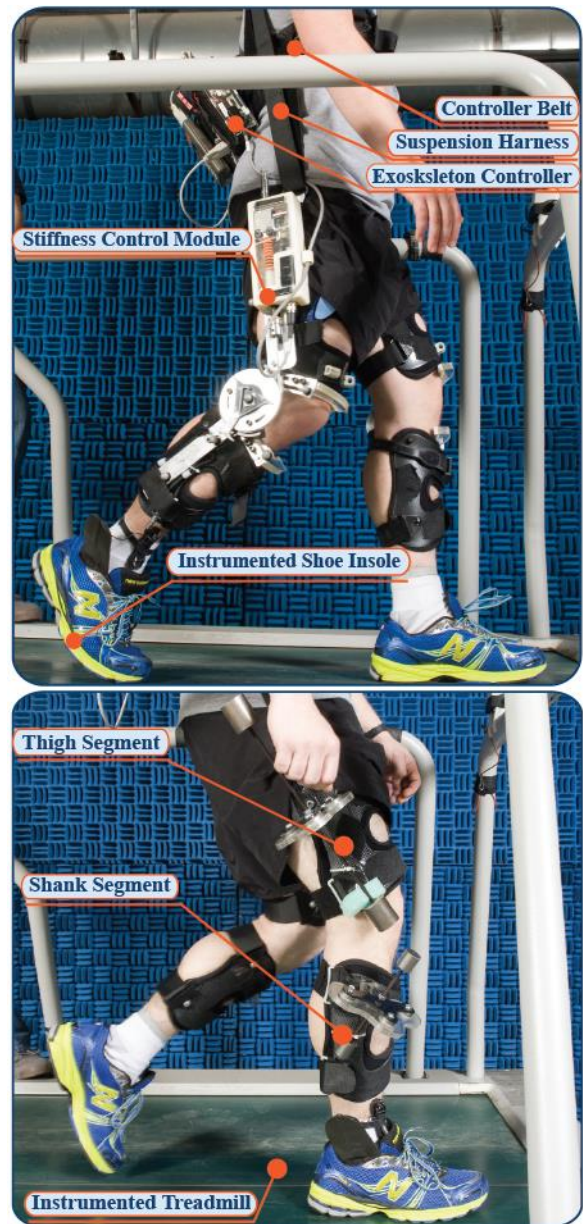
Fig. 3. Top: Quasi-passive knee exoskeletons worn on one of the participants during walking on an instrumented treadmill. Bottom: Joint-less mass replicas of the exoskeletons worn on a participant.
