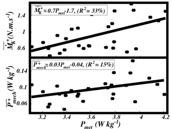
Fig. 4. Average positive rate of moment generation (top) and average positive power (bottom) with respect to the metabolic power. The graphs also include linear fits that show significant correlation ( $p < 0.01$  for the coefficients of the fit) between the parameters.
