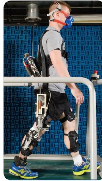
Fig. 1. The quasi-passive exoskeleton implements a spring in parallel with the knee joint in the weight acceptance phase and allows free rotation throughout the rest of gait cycle.
