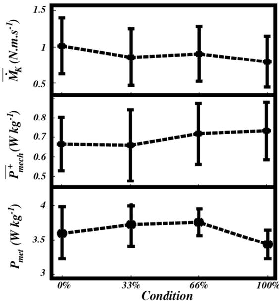
Fig. 3. Top: Average positive rate of moment generation for the knee joint, Middle: Average positive mechanical power of the knee, and Bottom: Metabolic power of walking across the experimental conditions. The error bars indicate  $\pm 1$  SD around the inter-subject mean values. The solid lines indicated the significant changes between the conditions.
