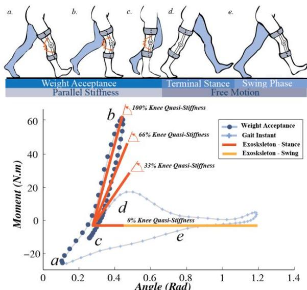
Fig. 2. Top: The exoskeleton implements a spring in the weight acceptance phase of the gait corresponding to the first ~40% of the gait cycle. Bottom: The experimental conditions involved walking with the exoskeletons with four levels of stiffness including 0%, 33%, 66%, and 100% of the estimated knee quasi-stiffness.
