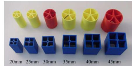
Fig. 9. Set of printed test objects used to evaluate the in-hand manipulation performance of the GR2 gripper prototype. The diameter/width varied between 20 and 45 mm. In all cases, the trakSTAR magnetic sensor was affixed to the object's center.
