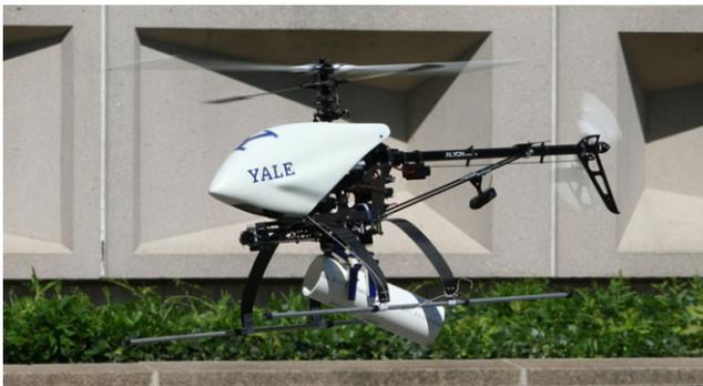
**Fig. 2** Yale Aerial Manipulator with gripper and fixed gear
