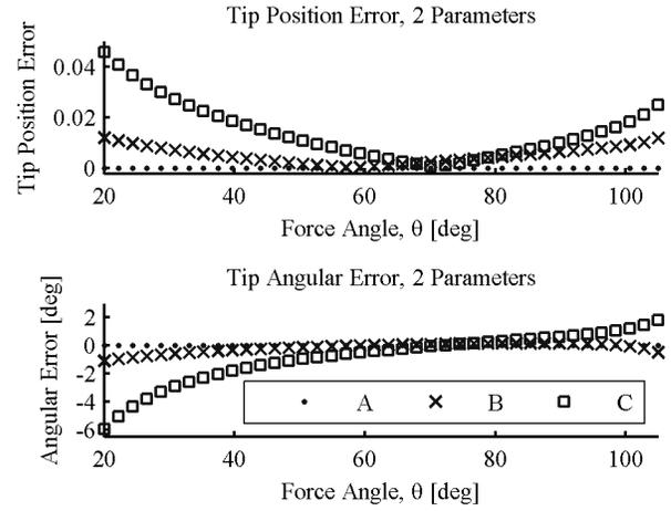
Figure 6. Prediction errors for the 2 parameter smooth curvature model. Cases A, B, and C correspond to the cases in Fig. 5.
