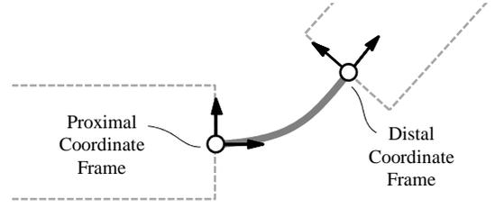
Figure 3. A Denavit-Hartenberg kinematic model of a flexure consists of a transformation mapping the coordinate frame at the proximal side of the joint to the coordinate frame at the distal side of the joint.
