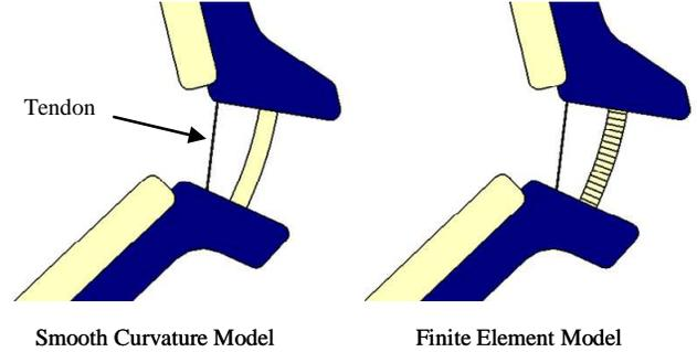
Figure 9. A single tendon-driven joint, modeled using the smooth curvature model (left) and finite rotational elements (right).
