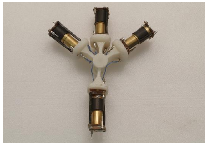
Fig. 4 Mechanical mates between cells and nodes. Multiple links (cells) can meet at a node. Each node mechanically acts as a pin joint.
