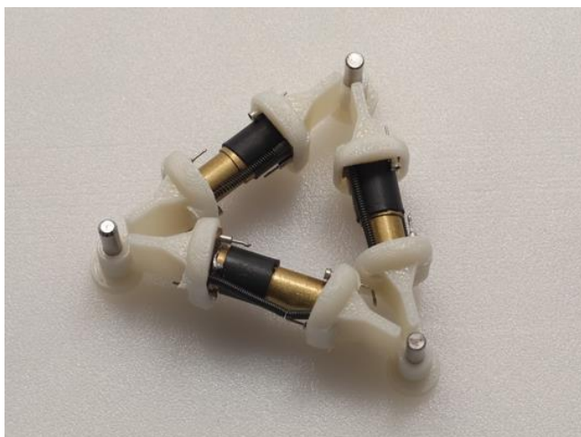
Fig. 6 Triangular active cell network: demonstrates the use of the pin joint (node) in the network to create planar structures.
