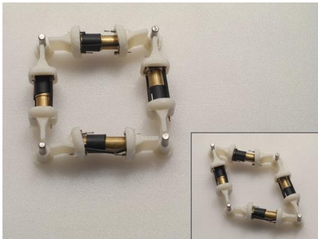
Fig. 5 Simple active cell network: square grid. Four nodes connect four links (cells). Activation of cells involves setting a potential difference between any pair of nodes. Inset shows alternative starting state.
