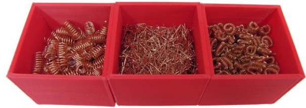
Fig. 3 Designs evaluated for the embedded cells: linear coils (left), copper filings (middle) and coiled-coils (right)
