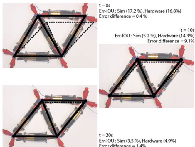
Fig. 11. A two-triangle MACRO mesh shape controlled to the specified target shape in simulation and in hardware (target shape shown in dashed lines; simulation output shown in solid lines). The shape-match error for the simulation and hardware trial (representative trial of five) is shown on the right.
