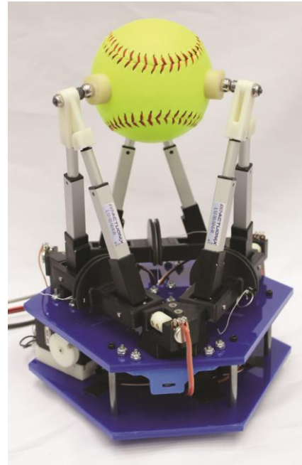
Fig. 1. The proposed parallel mechanism hand grasping a softball. All six prismatic actuators (used for 6-DOF manipulation) as well as the single revolute “grasp” actuator in the palm (used to close the hand) are easily visible.
