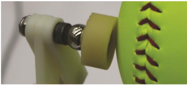
Fig. 6. Example of a fingertip rolling failure that was sometimes encountered near the limits of the workspace for certain manipulations. In these cases the object would roll on the fingertip rather than the spherical joint reconfiguring. Separation of greater than 4 mm was classified as a failure.
