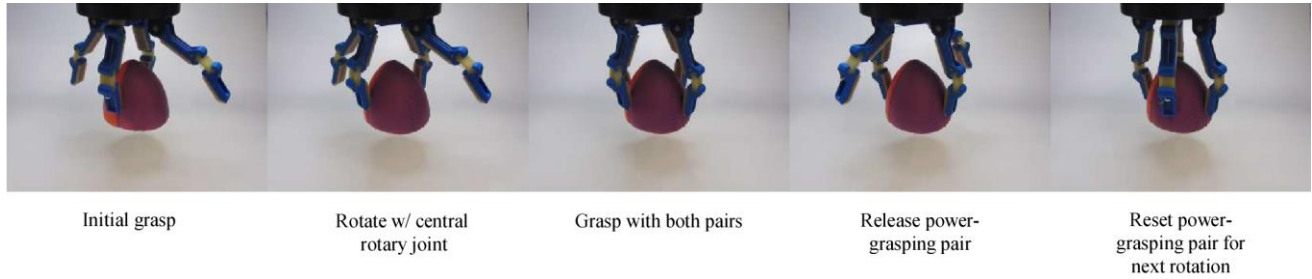
Figure 8. Example of an internal twisting manipulation primitive. Note that a grasp is maintained on the object at all times.
