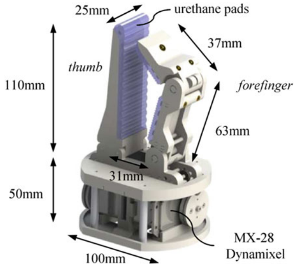
Fig. 1 Rendering of the proposed gripper with multiple operating modes. Weight of gripper is 430 g
