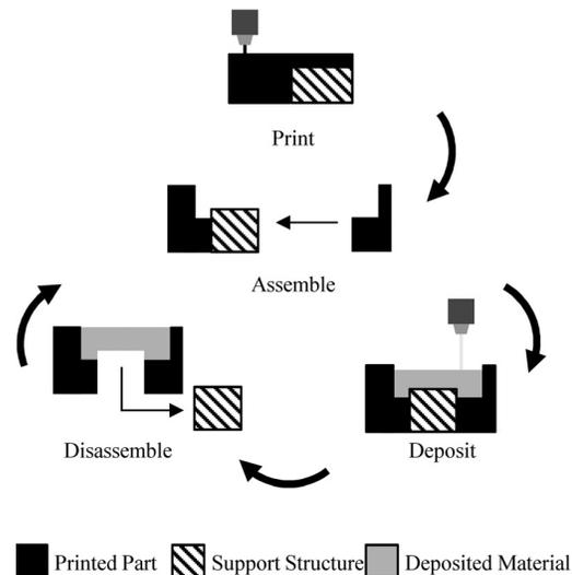
**Fig. 1 Summary of how 3D printing and resin casting can be combined to create novel mechanisms and structures through the HDM process, which may include multiple assemble-deposit-disassemble cycles**
