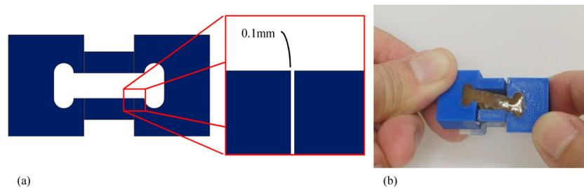
**Fig. 6 Regions printed side by side as separate contours can produce dissolvable or breakaway molds. In this example, the 0.1 mm gap separation is guaranteed to be smaller than the standard FDM printer's nozzle diameter (~0.4 mm). The optimal gap separation will depend on printer performance.**
