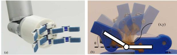
**Fig. 8** The OpenHand design (a) uses cast flexure joints and 3D-printed finger bodies and (b) tendons are routed across idler pins and pulleys to actuate the fingers. Its motion can be approximated as a revolute pin joint in certain configuration ranges.
