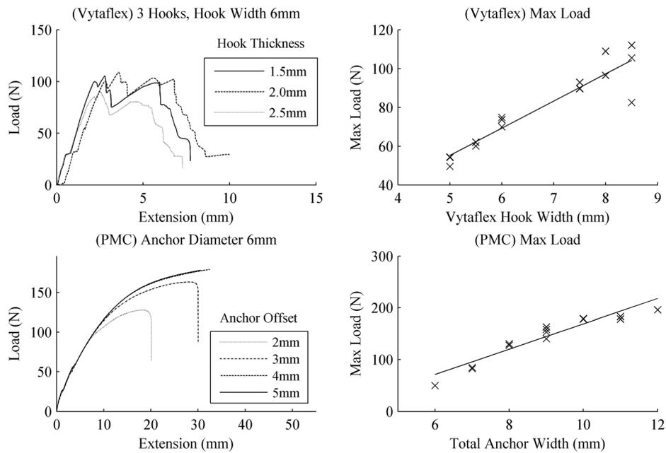
**Fig. 4 Tensile test results to determine failure points of various anchor designs. Results suggest maximizing the overall resin anchor protrusion size.**
