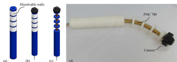
**Fig. 12** Example of a tendon-driven, snake-like camera probe. (a) The initial frame is printed with alternating solid (blue) and dissolvable (white) sections around a central core cavity, (b) the camera wires are positioned such that they route through the center core, and (c) The central core is filled with urethane, and the dissolvable sections are removed via the lye bath before the camera is attached.
