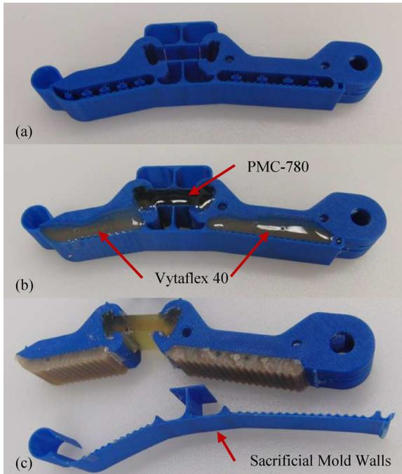
**Fig. 2** Steps to create an exemplar finger via the process described in this paper. (a) Mold component is printed with both sacrificial walls and core parts as a single monolithic part, (b) resin is deposited into the appropriate cavities, and (c) sacrificial features are removed with a file after deposited resins cure.
