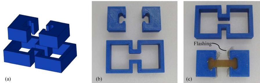
**Fig. 7 Example of snap-together, multipart molds that can be reused instead of destroying the temporary mold features**
