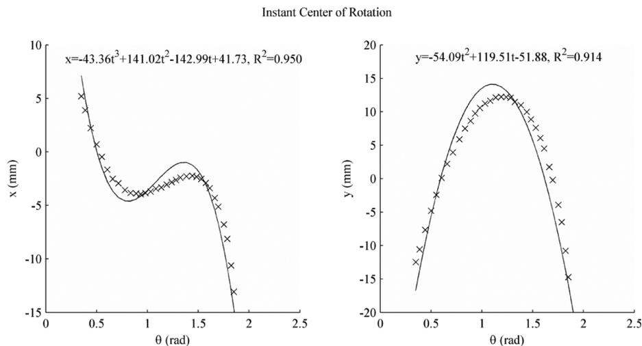
**Fig. 9** Flexure joints can be approximated as revolute joints under certain operating regimes. Buckling behavior of the flexure shifts its effective center of rotation at the upper and lower limits of its driving tendon's actuation space. Mechanisms utilizing flexural joints should be designed with this behavior in mind.
