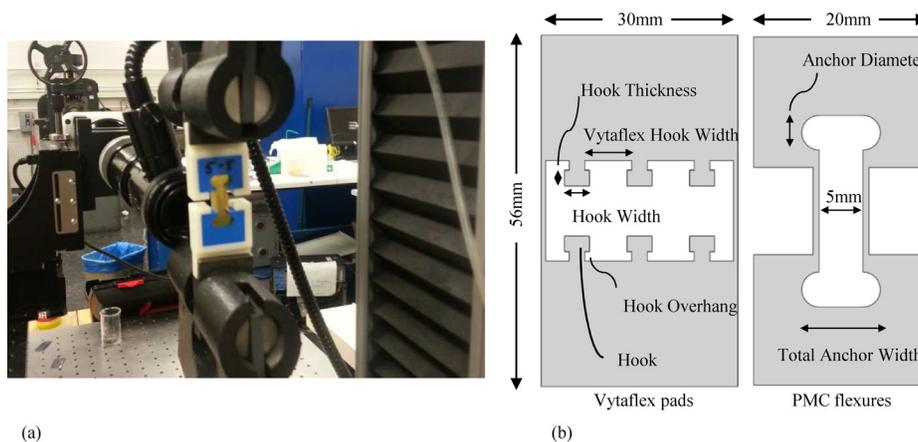
**Fig. 3** (a) Instron setup to test the tensile strength of various resin anchors in combination with printed ABS bodies and (b) parameters of the test samples for both Vytaflex 30 pads and PMC-780 flexures
