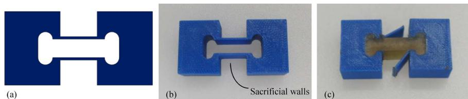
**Fig. 5 Mold cavity created with thin, sacrificial walls. The walls are manually removed, usually with a bandsaw or file, after the deposited resin cures.**
