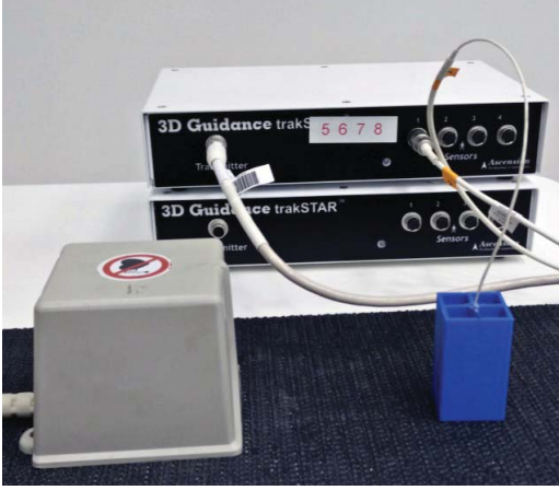
Fig. 9. TrakSTAR (Ascension Technologies) magnetic motion capture system and a rectangular sensorized, 3-D printed, rectangular object. The trakSTAR system is equipped with an MRT and 8 model-180 magnetic sensors that have a diameter of 2 mm. In this paper, we use a single sensor to capture the pose of the examined objects.
