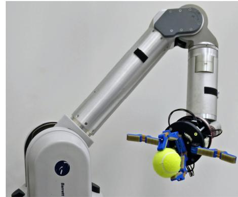
Fig. 6. The Barrett WAM - Yale model FG arm hand system, while grasping a tennis ball with a precision grasp.
