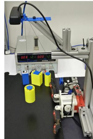
Fig. 4. The setup used for data collection. The frame is created with a set of T-slotted profiles of the Industrial Erector Set (80/20). The blue 3D printed camera holder has a pulley attached for repositioning the object (using the dedicated motor in the middle of the image). The red base of the hand is a 3D printed wrist coupling of the Yale Open Hand project [9].
