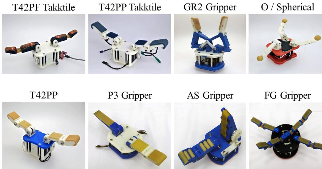
Fig. 3. The examined robot hands are depicted. All hands have been developed by the GRAB Lab at Yale University. Models T42 and O are freely distributed through the Yale Open Hand project website [9].
