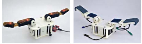
Fig. 5. The models T42PF and T42PP that are used in the experiments. The T42PF consists of a custom base and two fingers of the RightHand Robotics ReFlex hand [38] that are equipped with 8 tactile sensors. The T42PP consists of a custom base and two fingers with two spring loaded pin joints. Each distal phalanx is equipped with 5 tactile sensors.
