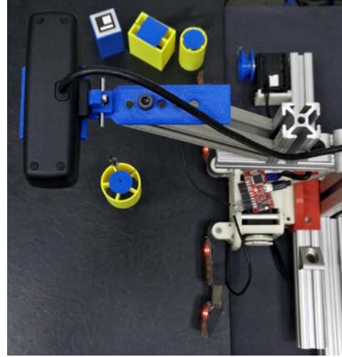
Fig. 6. The setup used for data collection. The frame is created with a set of T-slotted profiles of the Industrial Erector Set (80/20). A blue 3D printed base is used in order to hold both the web camera and a pulley for repositioning the object (using the dedicated motor at the top right side of the image). The red base of the hand is a 3D printed wrist coupling of the Yale Open Hand project [33].
