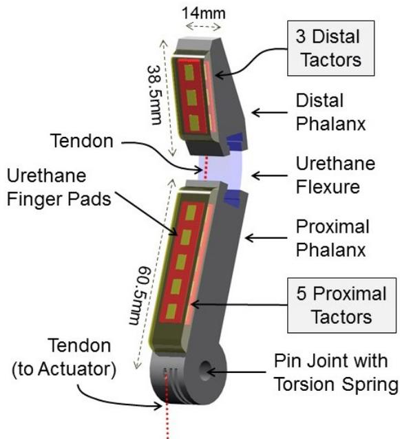
Fig. 2. The structure of an underactuated finger and the locations of the force sensors.
