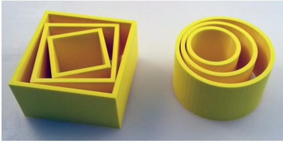
Fig. 4. The model objects of the first set. The boxes and cylinders have side lengths / diameters of 50, 70 and 90 mm.
