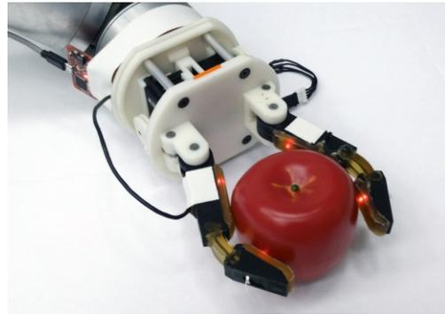
Fig. 1. A robot hand equipped with force sensors grasping a plastic apple for classification purposes.
