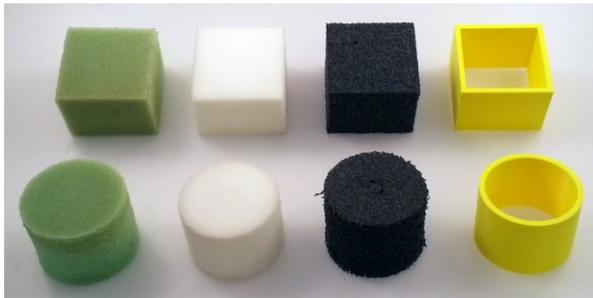
Fig. 5. The model objects of the second set. The first row depicts rectangles with same side length and different stiffness. The second row depicts four different cylinders with same diameter and different stiffness.
