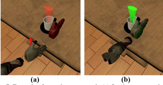
Figure 7. Example of a reach to a cup task. (a) Semi-transparent hand indicates the desired goal position of the user-controller hand, which dims as the hand approaches it. A red arrow is included next to the hand to assist with visualizing the current hand orientation. (b) Task completion occurs when the hand is within the Euclidean tolerance and the corresponding orientation arrow is within the tolerance cone.
