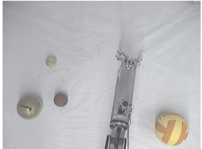
Fig. 13. Overhead image of the workspace showing the four target objects and the robot arm. Images of the workspace taken from this camera were used to find the target object location and size.
