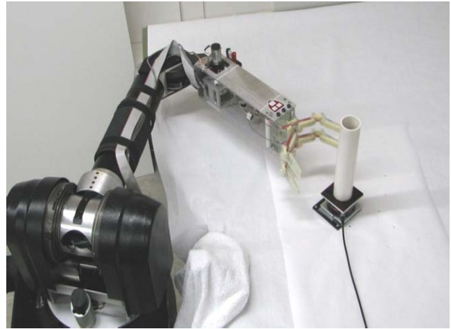
Fig. 7 Overhead view of WAM robot configuration. The table on the right half of the image is level with the ground and the arm operates in the plane until lifting the object
