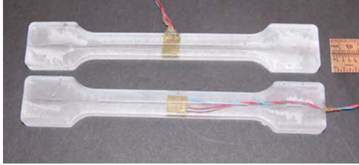
Figure 5.3. Metal film strain gages embedded in beam with side-exit wires (top) and axial-exit wires.
