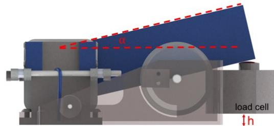
Figure 5. CAD rendering of the force output experimental setup. The angle,  $\alpha$ , above horizontal is the angle of the output link at impact.
