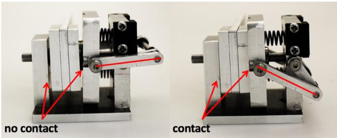
Figure 3. During normal operation (left) the lever is above horizontal, or zero degrees, and after collision (right) the lever is below. After collision the output link is pressed against the back plate and restricts movement.
