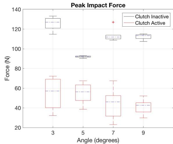
Figure 7. The graph displays peak impact force when the output link impacts a load cell at different link angles.
