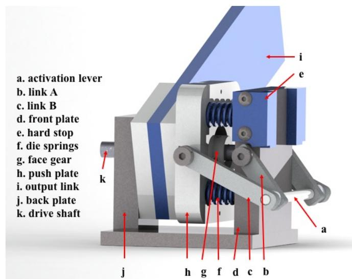
Figure 1. Annotated CAD rendering of the Fusion Clutch mechanism without the motor.
