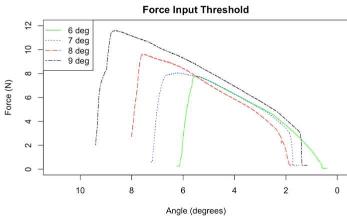
Figure 6. The graph displays force required to activate the mechanism versus angle of the lever. Zero degrees corresponds to the horizontal position or singularity point of the activation lever.
