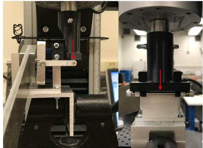
Figure 4. Force input testing. The arrow shows direction the Instron applies force on the activation lever.
