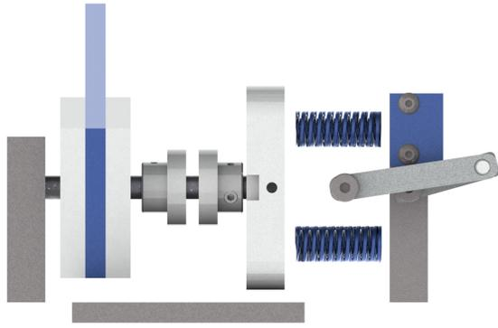
Figure 2. Exploded view of Fusion Clutch. The face gear on the left is securely attached to the output link, and the face gear on the right is coupled with the drive shaft.
