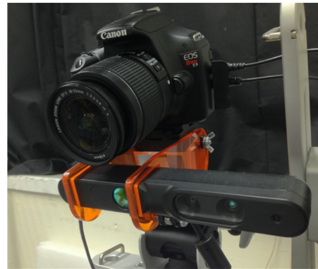
Fig. 1. A Canon Rebel T3 RGB camera and PrimeSense Carmine 1.08 RGB-D sensor pair mounted together.
