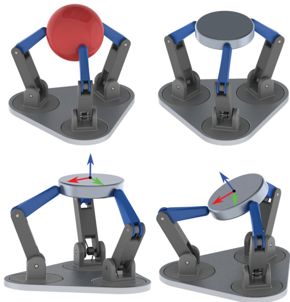
Fig. 1. Top: A simple three-fingered hand doing two tripod precision grasps. Bottom: Two in-hand object poses. We want to explore how to optimize the geometry of the hands to maximize the number of in-hand object poses that can be achieved during in-hand manipulation without breaking contact.
