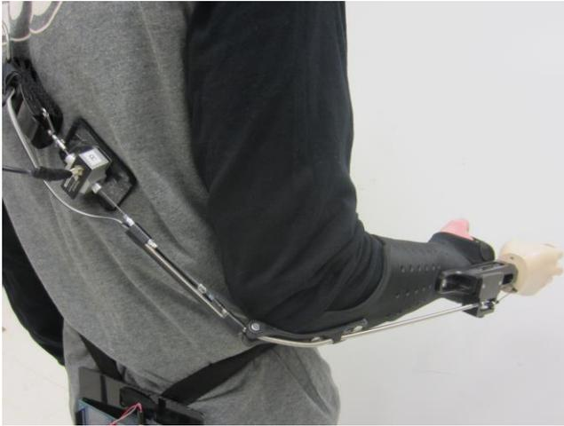
Fig. 6. An instrumented bypass socket was used to evaluate the body-powered terminal devices with able-body subjects. Here, the subject is using the APRL voluntary-closing hand with a standard figure-of-nine harness.
