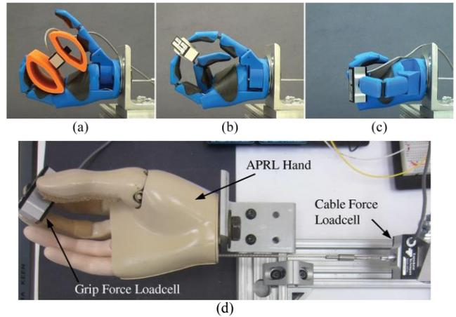
Fig. 3: Grip force measurements of the Yale Multigrasp Hand, a) power grasp configuration with the orange grasp cylinder to simulate larger cylindrical objects, b) precision grasp where the grip force is strictly between the index finger and thumb, and c) lateral grasp between the thumb and the side of the index finger. d) The same test performed on the APRL hand.
