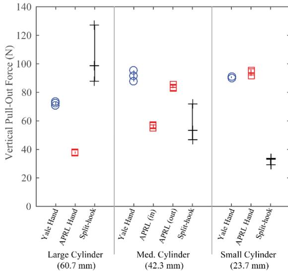
Fig. 4: The vertical pull-out force was measured for the Yale and APRL hands with a constant 75 N input force on the voluntary-closing body-powered cable. The Hosmer Hook was tested with no load on the body-powered cable (the scenario which produced the largest grasp force).
