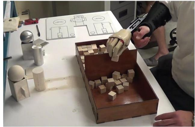
Fig. 7. An able-body subject performs the Box and Blocks test with the APRL and the by-pass socket.
