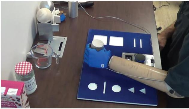
Fig. 8. An amputee subject uses the Yale Multigrasp Hand to complete the SHAP test. Here, the subject is manipulating the Heavy Cylinder abstract object.
