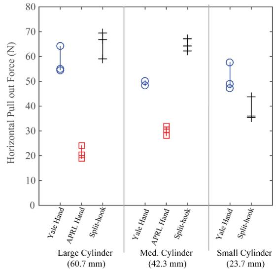
Fig. 5: The horizontal pull-out test was performed by pulling on three different sized PVC cylinders in the direction that slid them out of the grasp from the side (the white cylinders were pulled upward in the images above). This test is similar to the NIST “Slip Resistance” test [10]. Here, images are shown for the Yale Hand, the APRL Hand, and the Hosmer Split-hook. The APRL Hand was unable to close on the small cylinder.
