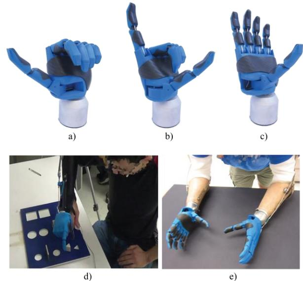
Fig. 1. The Yale Multigrasp Hand features lateral (a), precision (b), and power grasps (c) all actuated through a single body-powered cable. The grasp type is selected through a simple movement of the thumb. The hand was evaluated by able body subjects, (d) as well as amputees (e).
