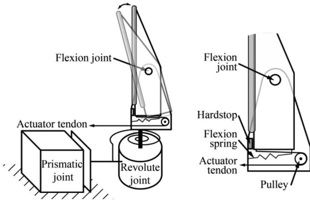
Fig. 2. Diagram of the finger kinematics (left) and detailed view of the flexion mechanism (right). Each finger consists of an actuated prismatic joint, an unactuated revolute joint with return spring, and a finger with an actuated flexion joint. The extension of the flexion joint is limited by a mechanical hard stop and achieved via a spring.
