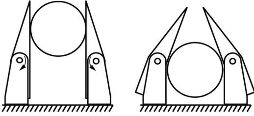
Fig. 6. Diagram showing the side view of the flexor behavior of the fingers. When performing either a spherical or cylindrical grasp, once the fingers make contact, the actuated flexion degree of freedom causes the fingers to wrap about the object (left), resulting in a more secure grasp as shown (right).
