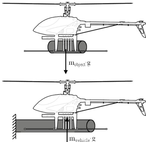
Figure 2. Diagram showing a helicopter carrying an object (top) and perching (bottom). When carrying the object, the hand has to resist a downward force to the object to oppose the objects mass. In contrast, when perching, the hand has to transmit an upward force from the perch to the vehicle.
