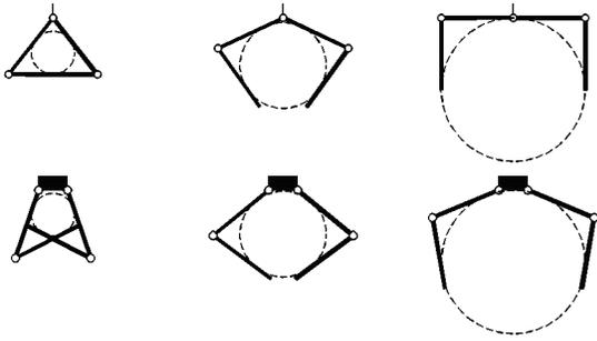
Figure 5. Examples of grasps for various object diameters and palm widths. Since all lengths have been normalized by the total length of the two digits, the object diameter and palm width are expressed relative to this length and are unitless. The left column shows 0.1 diameter objects, the middle 0.3, and the right 0.5. The first row shows hands with a palm width of zero while the second row shows hands with a palm width of 0.1
