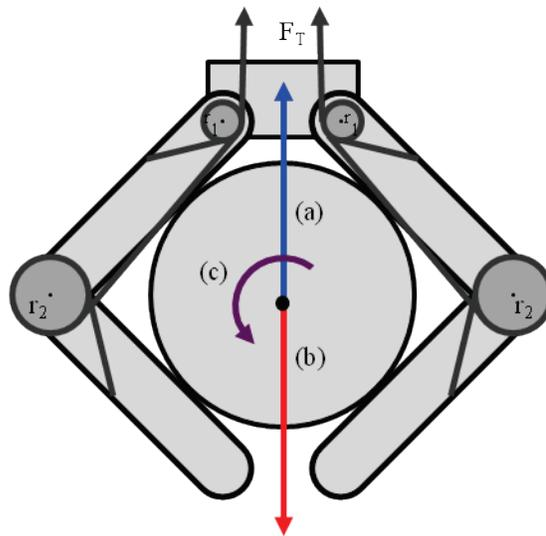
Figure 3. Diagram of hand showing proximal and distal tendons and example of upward or palmar disturbance force (a), downward disturbance (b), and moment disturbance (c).
