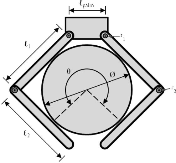
Figure 4. Example of manipulator wrapped about a circular object. Hand and object parameters including wrap angle,  $\theta$ , object diameter,  $\phi$ , proximal link length  $\ell_1$ , distal link length  $\ell_2$ , palm length  $\ell_{palm}$ , proximal pulley radius  $r_1$  and distal pulley radius  $r_2$  are shown.
