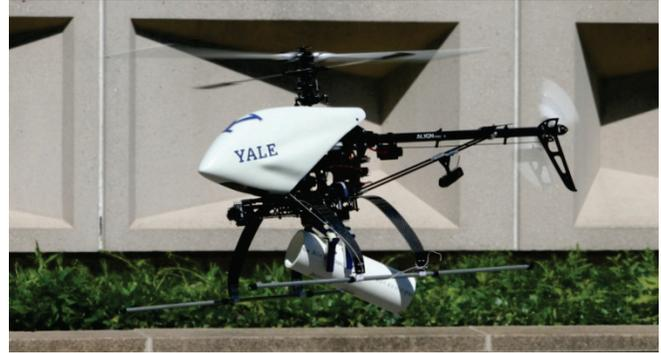
Figure 1. Example of a UAV grasping and carrying an object using an underactuated hand [10].
