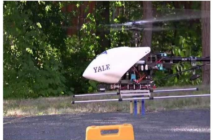
**Figure 1. Example of a UAV preparing to grasp an object while in flight.**
