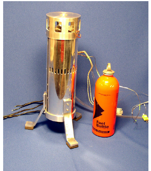
Fig. 7. Picture of the first generation integrated system with separate fuel tank.
