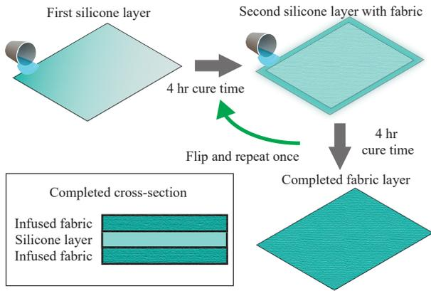
Fig. 4. Fabrication of the silicone-infused double-layer fabric (SIDF).
