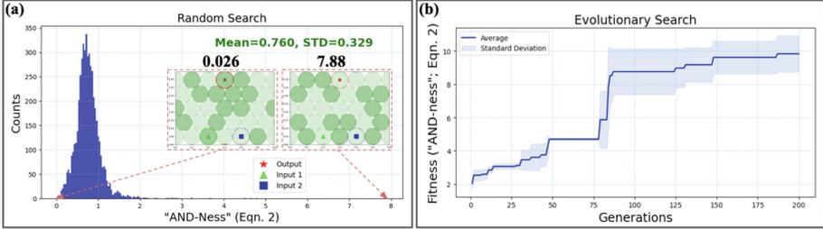
**Fig. 6.** Designing an AND gate in a stiffness-contrasting assembly of particles. (a): The histogram shows the distribution of “AND-ness” in 5000 random configurations, as well as the best and worst material found. Light and dark green colors indicate soft and stiff particles, respectively. (b): The plot shows the progress of optimization during 200 generations. (Color figure online)
