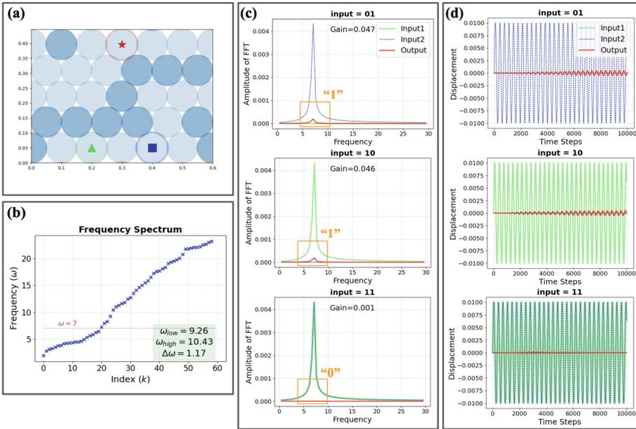
**Fig. 10.** One of the best designs for an XOR gate found for materials with mass-contrasting particles. (a) and (b) report the evolved configuration and its band gap features. (c) reports the material’s response at the driving frequency (7) and all other frequencies. (d) shows material’s behavior over time when presented with three of the four input cases.
