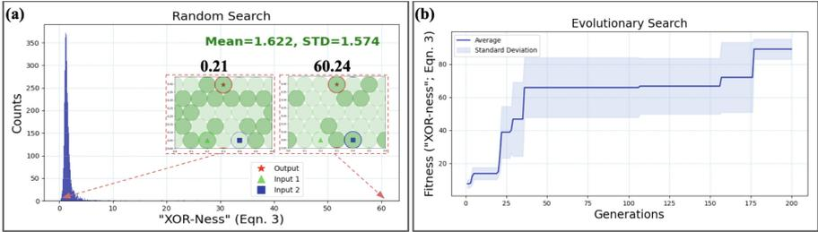
**Fig. 12.** Evolving XOR behavior into a stiffness-contrasting assembly of particles. (a): The distribution of XOR-ness (as defined in Eq. 3) in 5000 materials found by random search. (b): Average performance of the three evolutionary trials.
