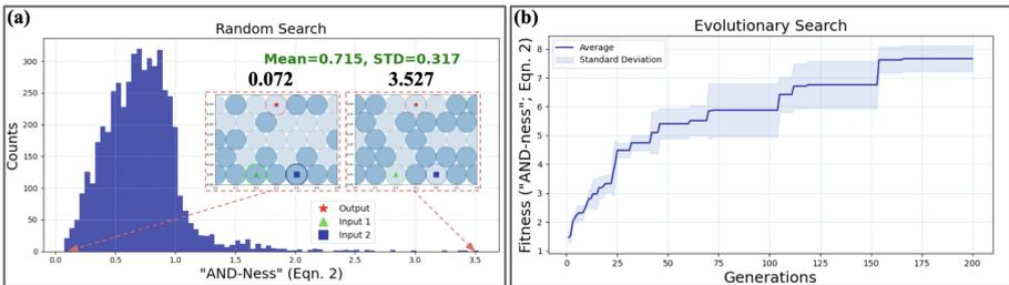
**Fig. 3.** Designing an AND gate in a mass-contrasting assembly of particles. (a): The histogram shows the distribution of the AND-ness in 5000 random configurations. (b): The plot shows the progress of optimization during 200 generations.
