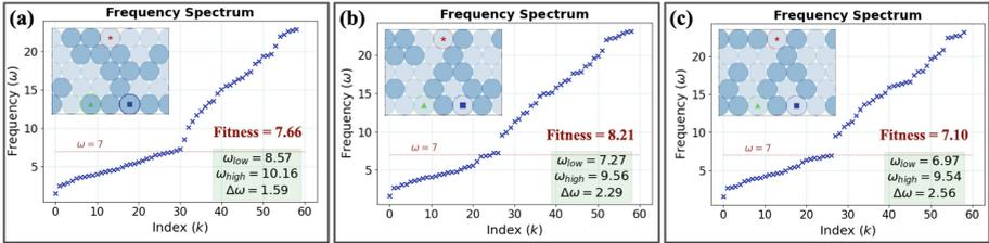
**Fig. 5.** The fittest AND gate designs from the three evolutionary trials, using mass-contrasting particles. Their frequency spectra, band gap features, and fitness values (Eq. 2) are also shown.
