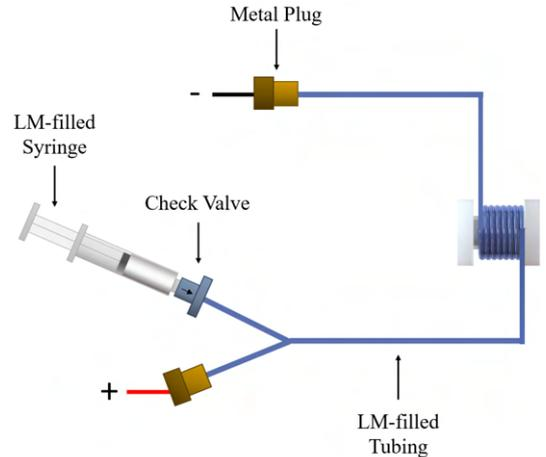
Fig. 3. Diagram of the fluidic circuit designed to mitigate the effects of electromigration. The tubes filled with liquid metal (LM) that make up the electromagnetic coil extend to two metal plugs to which wire leads were attached. LM was injected using a syringe until the tubes were filled, and then the tubes were capped with the metal plugs. A check valve was used to prevent back flow into the syringe.
