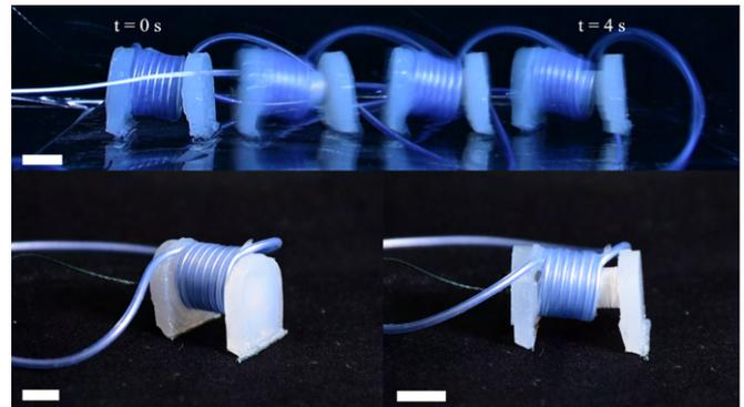
Fig. 1. An example locomotion trial. The robot achieves locomotion by repeatedly attracting and repelling an on-board permanent magnet. Scale bars: 1 cm.
