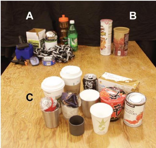
Fig. 5. Objects used to evaluate the classifier. (A) and (B) were used to test a stationary gripper, while (C) were objects used in the full recycling setup. The objects in (A) were successfully classified while the objects in (B) were unsuccessfully classified.
