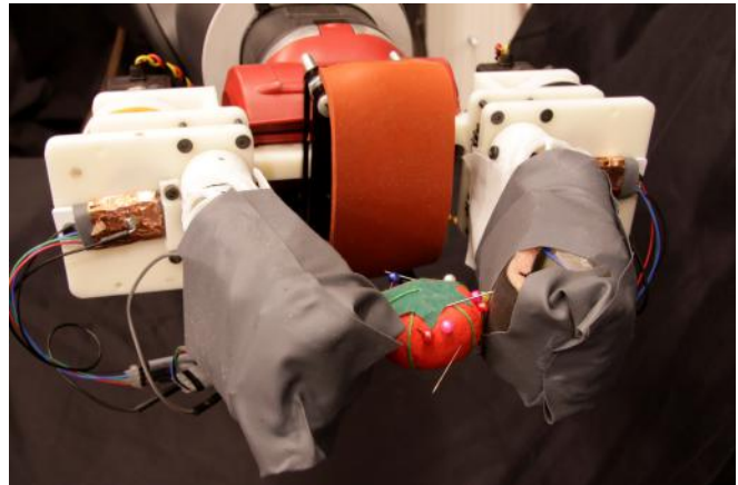
Fig. 1. Demonstration of the soft robotic gripper holding a spiky pincushion, demonstrating its resistance to puncture and lacerations. Each finger of the soft robotic gripper is made of a pair of handed shearing auxetic cylinders and high-deformation capacitive pressure and strain sensors. The gripper can grasp objects and detect their base material without fear of sharp objects.
