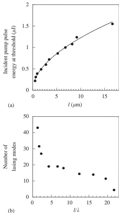
Fig. 1. (a) The incident pump pulse energy at the lasing threshold versus the transport mean free path. (b) The number of lasing modes versus the transport mean free path.
