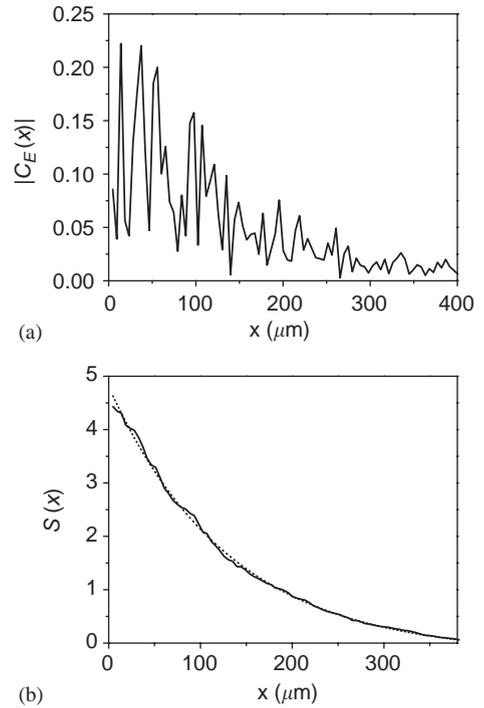
Fig. 2. (a) The amplitude of spatial field correlation function  $C_E(x)$  for a lasing state. (b) The solid line is  $S(x)$  obtained by integrating  $|C_E(x)|$  in (a). The dotted line represents the fitting of an exponential decay function.
