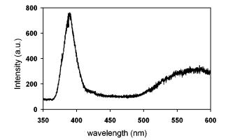
FIG. 4. PL spectrum of 202 nm ZnO inverted opal. This sample has no band gaps overlapping the emission spectrum.
