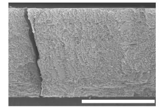
FIG. 1. SEM of a cleaved cross section of a 255 nm ZnO inverted opal structure (scale bar equals 20  $\mu$ m).
