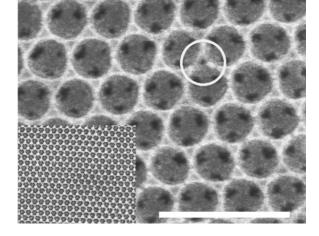
FIG. 2. SEM image of exposed (111) top surface of 356 nm ZnO inverted opals (scale bar equals 1  $\mu$ m). The interstitial pores inherent in the infiltration process remain open after firing of the structure (circle). Inset: Lower magnification image of (111) surface. Downloaded 10 Apr 2005 to 129.105.151.28. Redistribution subject to AlP license or copyright, see http://apl.aip.org/apl/copyright.jsp
