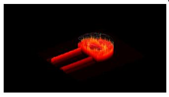
The D-shaped cavity producing quantum chaos within the cavity, and a more stable laser resulting. Credit: Bittner et al.
