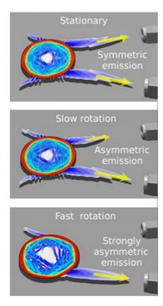
These are schematics showing the far-field emission pattern of a microdisk cavity changing from symmetric to strongly asymmetric. Two cameras on the right monitor the change. Credit:Li Ge, physicist at the Graduate Center and Staten Island College, City University of New York
