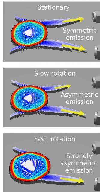
These are schematics showing the far-field emission pattern of a microdisk cavity changing from symmetric to strongly asymmetric. Two cameras on the right monitor the change.
