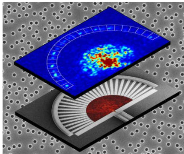
*Yale University researchers have developed an ultra-compact, low-cost spectrometer with improved resolution over existing micro models. The innovation represents an advance in "lab-on-a-chip" technology, or the consolidation of laboratory capabilities in miniature, highly portable devices.*
