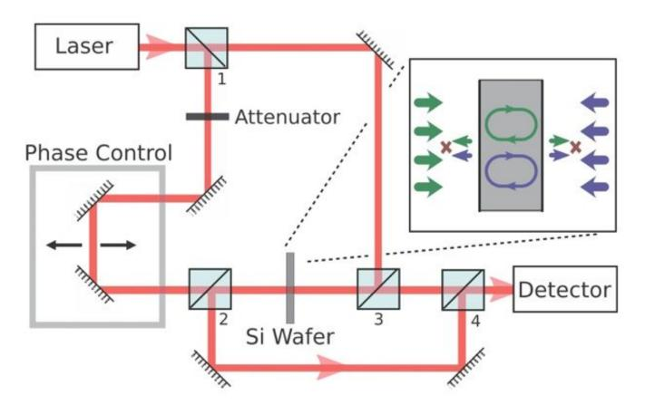
When the alignment was right, the light waves canceled each other out. The silicon absorbed the light and converted it to another form of energy, like heat or electrical current.
