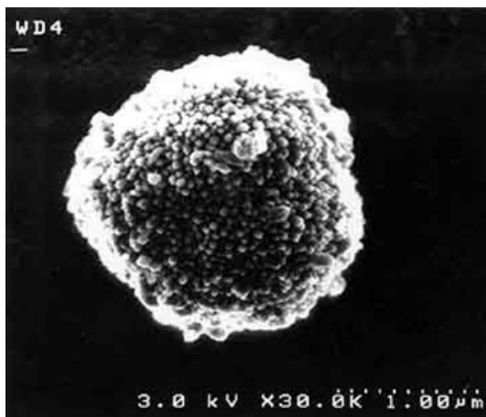
Scanning electron microscope photo of a micron-sized zinc selenide particle used in a powder laser. (Source: Northwestern University)
