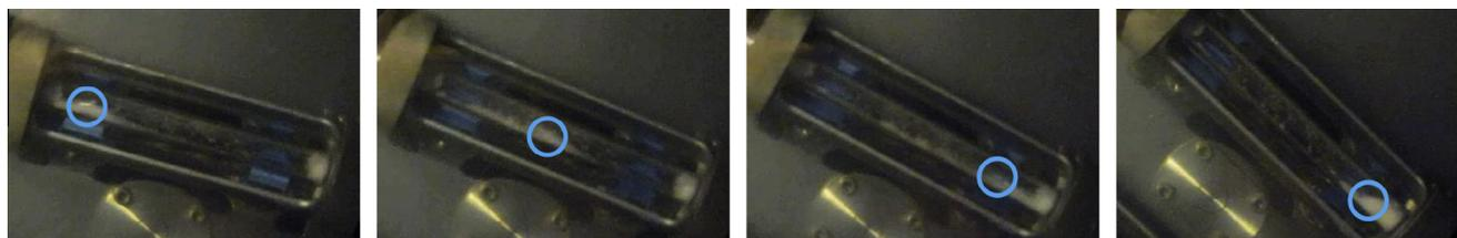
**Fig. 2.** Hydrate Test 12 (Gas 1). Images of hydrate powders movement along the steel ball during rocking test. Images are taken at 8.5 °C and 88 bar. The process happens in less than 1 s. The blue circle shows the positions of steel ball. (For interpretation of the references to colour in this figure legend, the reader is referred to the web version of this article.)
