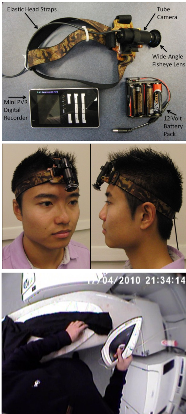
Fig. 2. Camera and receiver hardware (top), example of the apparatus as worn by a subject (middle), and sample image from the system in use.
