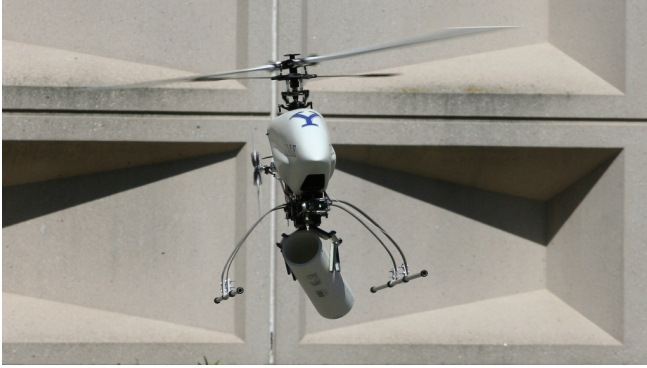
Figure 1. AERIAL MANIPULATION TESTBED CARRYING A TUBE.
